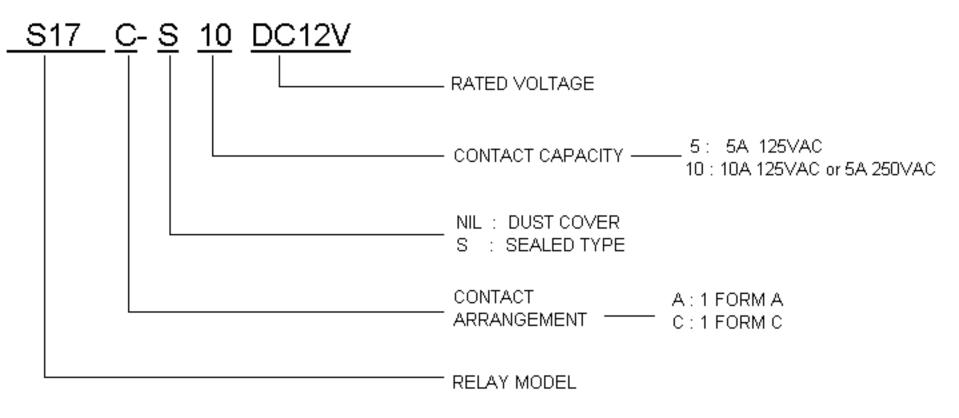
(i.e. S17C-S10-DC12V is a SPDT, 10Amp, fully sealed, 12VDC coil relay.)
